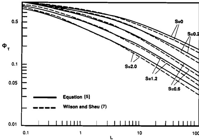
Fig. 2—Comparison of thermal reduction factors as predicted by Eq. [5] and the Wilson and Sheu formula (7).
