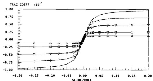
Fig. 5—Traction prediction of Type II viscoelastic model as a function of the limiting shear stress.
