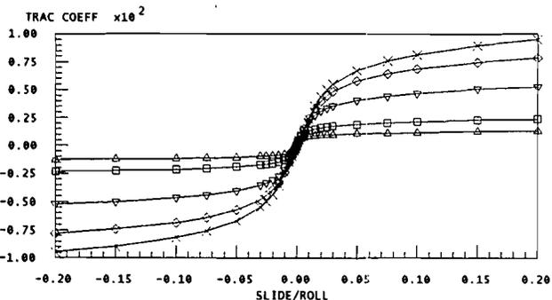
Fig. 4—Traction prediction of Type I viscoelastic model as a function of critical shear stress.
