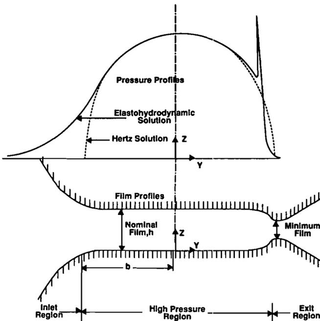
Fig. 1—Schematic representation of an elastohydrodynamic contact zone.
